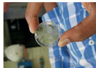
Fig. 5: Optical window contaminated by sulphur.
