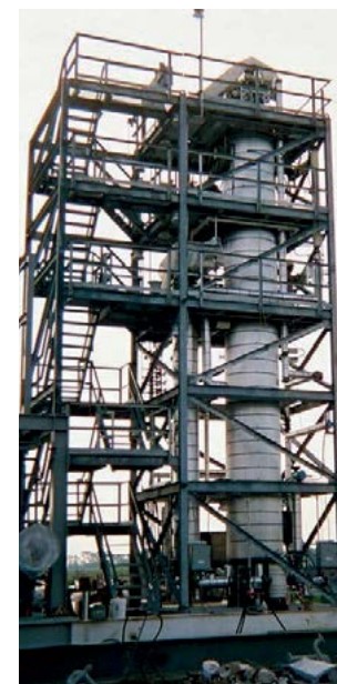
Truckable module with contactor, cooler and major controls. Up to 800 t/d liquid sulphur processing capacity.
