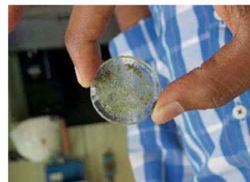
Fig. 5: Optical window contaminated by sulphur.
