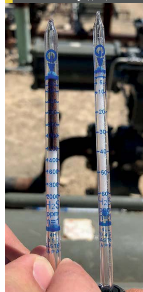
Fig. 9: GasTec tubes – sour gas in, sweet gas out (black indicates H 2 S ppmv)
