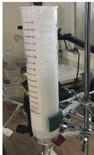
Fig. 3: Foam Test of Black Powder Solvent added to Amine Solvent.
