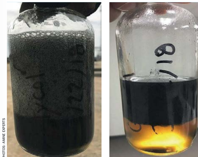
Fig. 1: Lean TEG sample showing foam (left) and with phase separation 24 hrs later (right).
