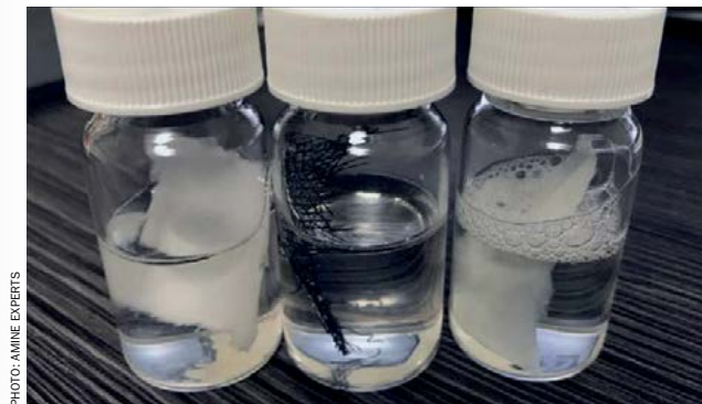
Fig. 4: Soak and foam test of the materials in the lean amine filter using fresh 50% formulated MDEA. Test was performed at 77°F for 4 hrs. The vials were agitated for 1 minute. The image was taken after 5 min resting. Left: cotton media (no foam formation). Middle: filter support screen (no foam formation). Right: white cellulose media (high foam formation and high foam stability).
