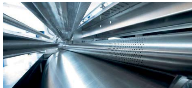
A view inside the Rotoform machine, showing the deposition cylinder and steel water-cooled belt.
