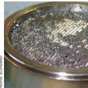
Residue on filter mesh.
