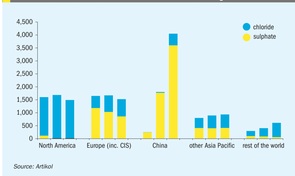
Fig. 1: TiO 2 capacity, by region: sulphate vs chloride (end-year capacity, 1999-2009-2019, in '000 t/a TiO 2 )
