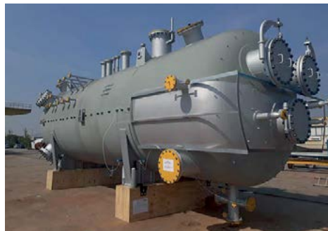
Fig. 5: New waste heat boiler (rear view)
