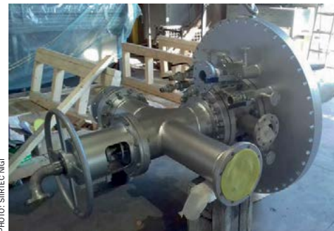
Fig. 4: Oxygen enrichment Claus burner
