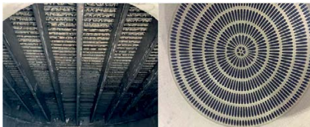
Fig. 2: Acid tower packing support. Project A (left): metallic support. Project B (right): self-supported ceramic dome.
