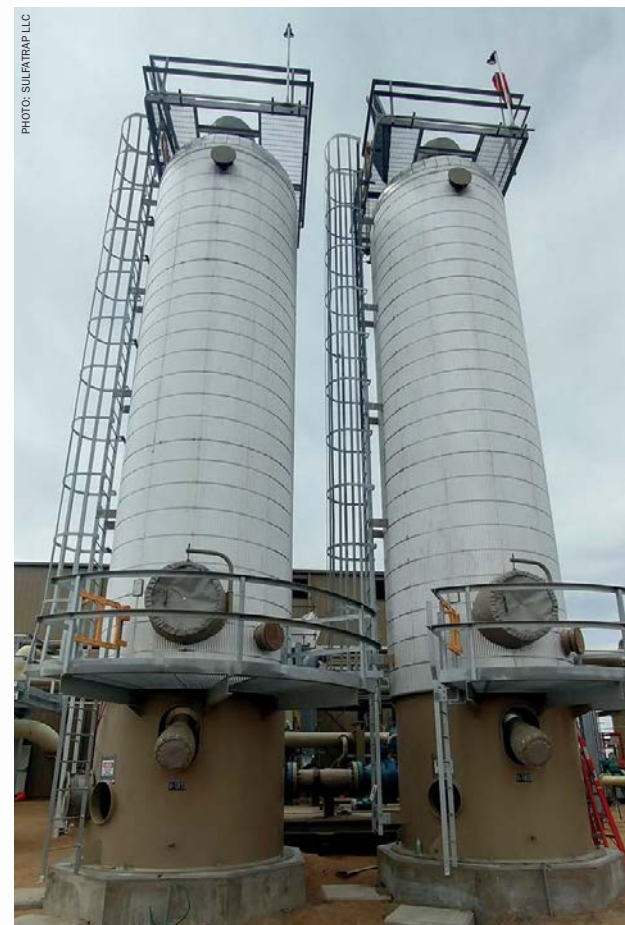
A lead-lag system treating compressed natural gas, designed and fabricated by SulfaTrap LLC.
