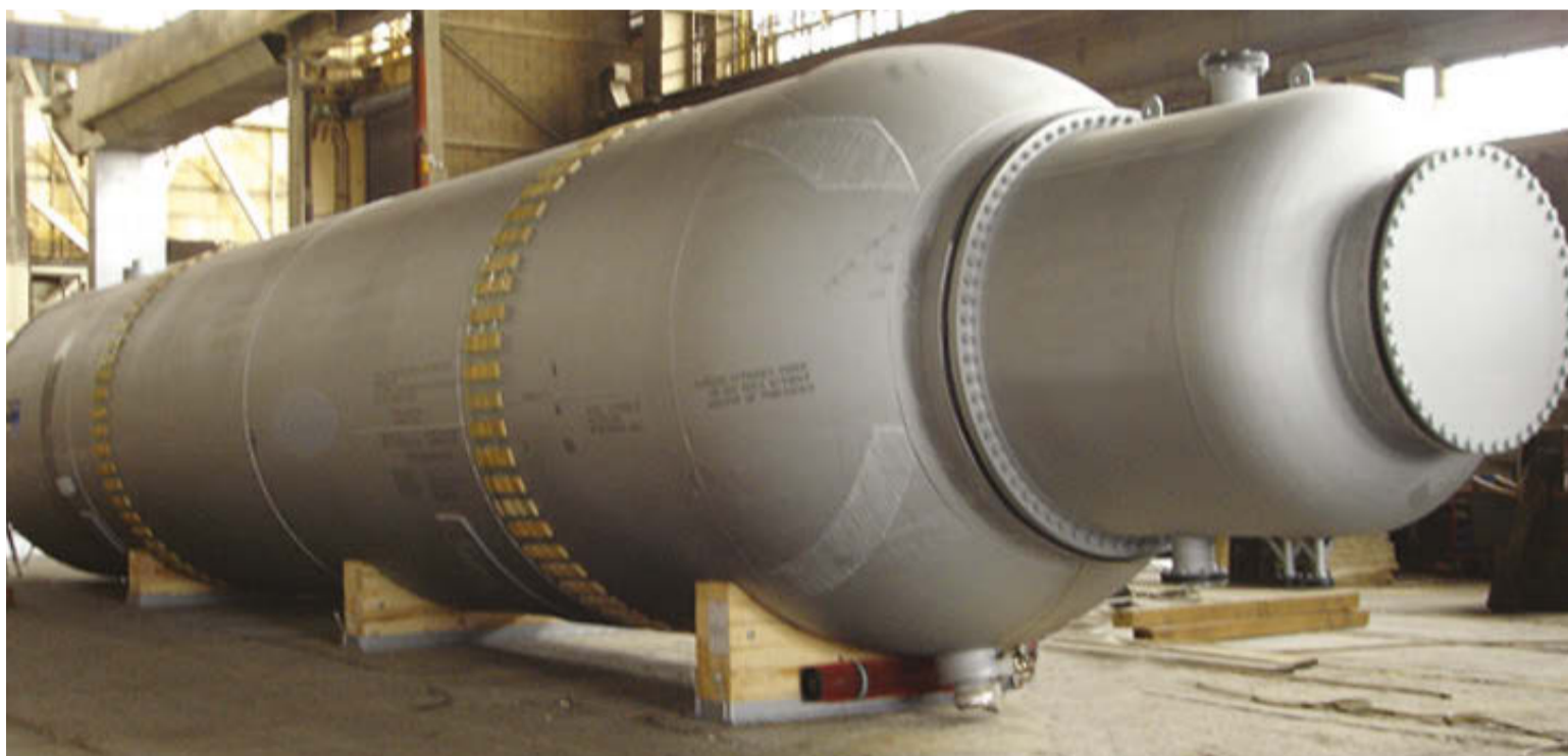
Fig. 1: Pool Reactor (NX STAMI Urea™) made with Stamicarbon's E-type super duplex stainless steel.
