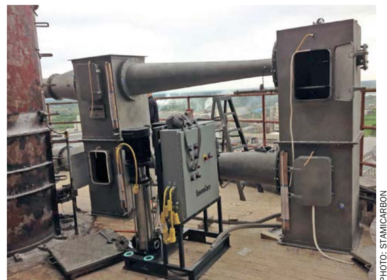
Fig. 9: Pilot Jet Scrubber located on top of prilling tower for emissions testing.
