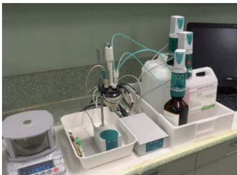
Fig. 1: Apparatus for the rapid determination of P 2 O 5 in phosphoric acid by thermometric titration.
