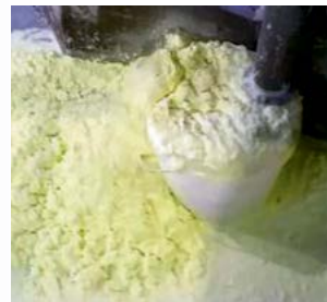
Fig. 2: Hydrophobic sulphur particulates floating in scrubbing liquor
