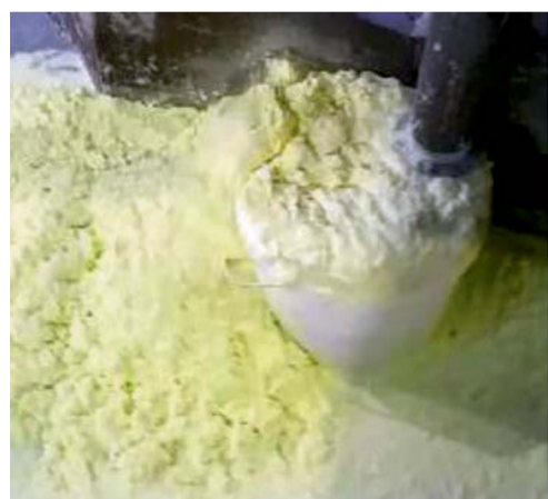
Fig. 2: Hydrophobic sulphur particulates floating in scrubbing liquor
