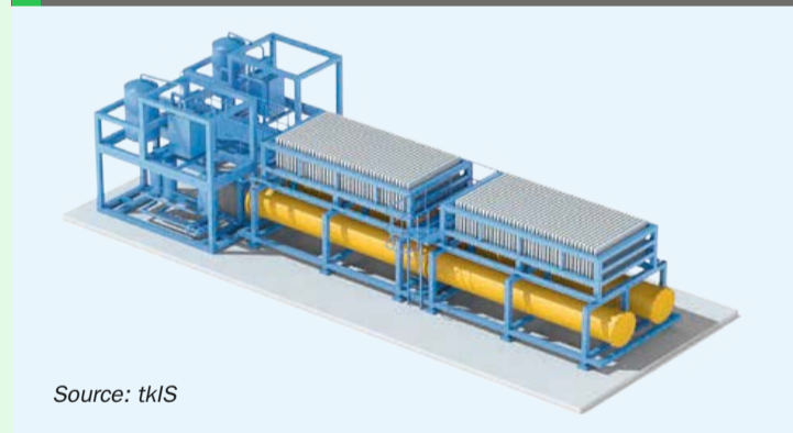
Fig. 6: 3D model of 5 MW electrolysis skid
