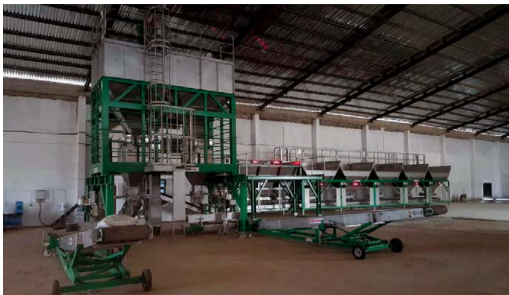
EMT Weighcont blender and bagging machine at a fertilizer blending factory in Ghana.
