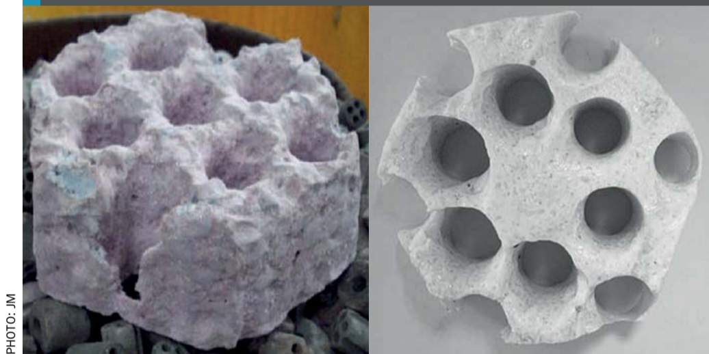
Fig. 8: Examples of alumina target tile erosion after service
