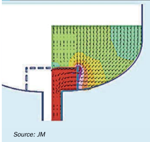
Fig. 10: STREAMLINE flow modelling of shift reactor
