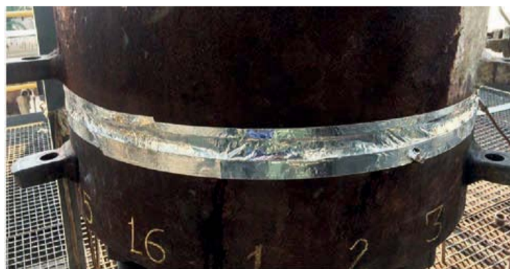
Fig. 3: Tightness test for large size flanges.
