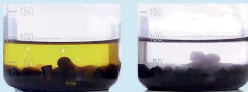
Fig. 18: Chromium VI visible in ShiftMax 120 (L); absent in ShiftMax 120 HCF (R)
