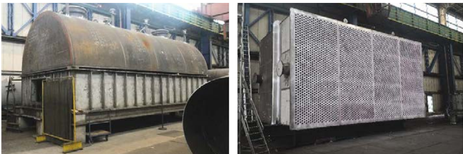
Fig. 6: CORE™ reactor under construction: top and bottom vestibules (left), central tube section (right)
