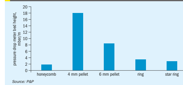
Fig. 3: Comparison of pressure drop for PPH catalysts and various shapes of vanadium pentoxide catalysts (indicative values)
