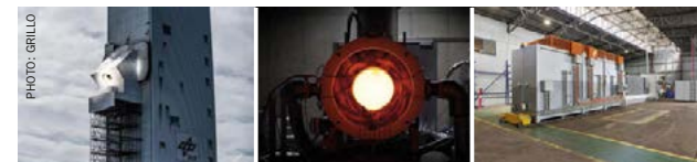
Fig. 8: High temperature industrial renewable heat possibilities for catalytic sulphuric acid splitting, left: CentRec solar receiver at the DLR solar tower in Juelich 27 , middle: Synhelion solar receiver 28 , right: SiBox module for latent heat thermal energy storage 29 .
