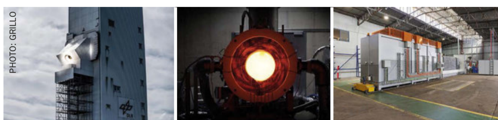
Fig. 8: High temperature industrial renewable heat possibilities for catalytic sulphuric acid splitting, left: CentRec ® solar receiver at the DLR solar tower in Juelich 27 , middle: Synhelion solar receiver 28 , right: SiBox ® module for latent heat thermal energy storage 29 .
